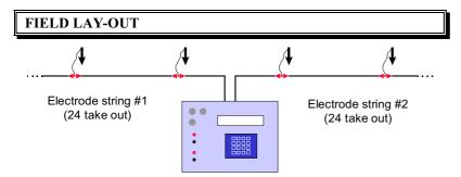
Preset arrays (Wenner, dipole,...) or customized arrays are uploaded through the user-friendly ELECTRE (version 2) PC software. The roll-along capability is implemented.
