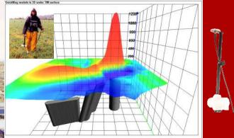
Single sensor and gradiometer modes provide flexibility and fast sampling and are used for detecting changes in the magnetic field. Applications include; alteration mapping, structural geology, archeology and UXO applications
