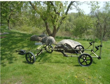
This image of a cart-borne system shows a simple 2 sensor array in operation.
